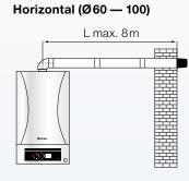
Horizontal connections L max. 8 m (including 90° elbow) Vertical connections L max. 9 m
