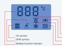
Burner burning symbol Fault warning indicator Frost protection Pre-heating
