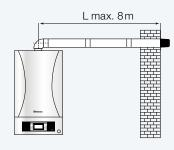
Horizontal connections L max. 8 m (including 90° elbow) Vertical connections L max. 9 m
