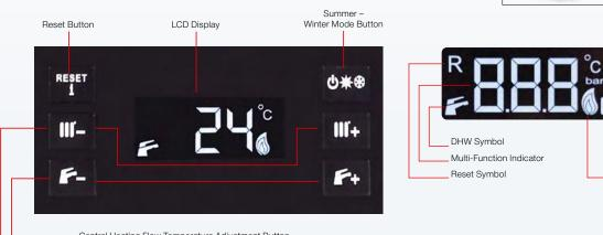
Fault Warning Indicator Burner ON Symbol
